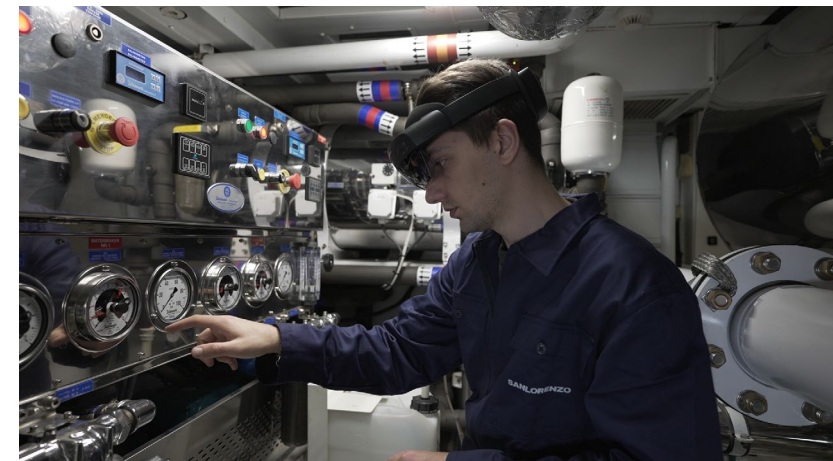
The Smart Helmet , developed by Sanlorenzo R&D department to provide timely remote assistance services to crews
