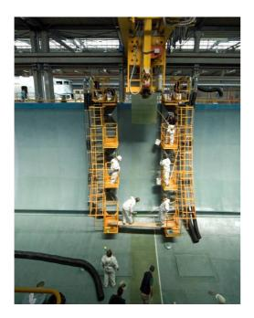
The superstructures are built in a "sandwich" configuration (two layers in fibreglass and carbon fibre encasing an internal balsa layer) with the vacuum infusion method, already successfully used by Intermarine to build 13 m patrol boats and for the bridges of 28 and 36 m patrol boats, but employed for the first time for minehunter superstructures.
