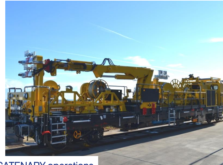
Innovative railcar for CATENARY operations
