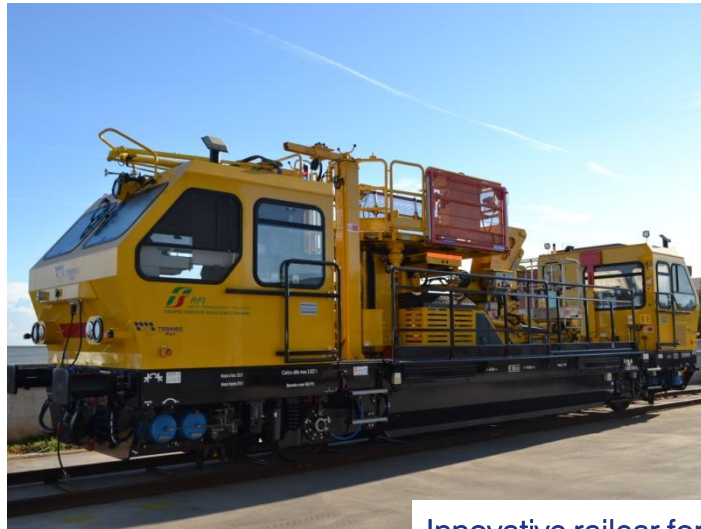
Innovative railcar for CATENARY operations
