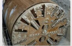
**DRILLING / TUNNELING**Tunnel-boring machines
