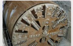
**DRILLING / TUNNELING**Tunnel-boring machines
