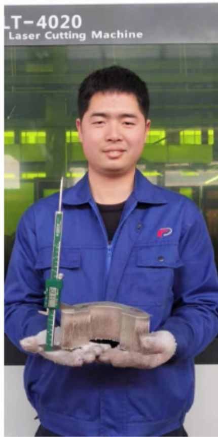
73mm stainless steel, another break-through cut by PENTA's 15kW.
