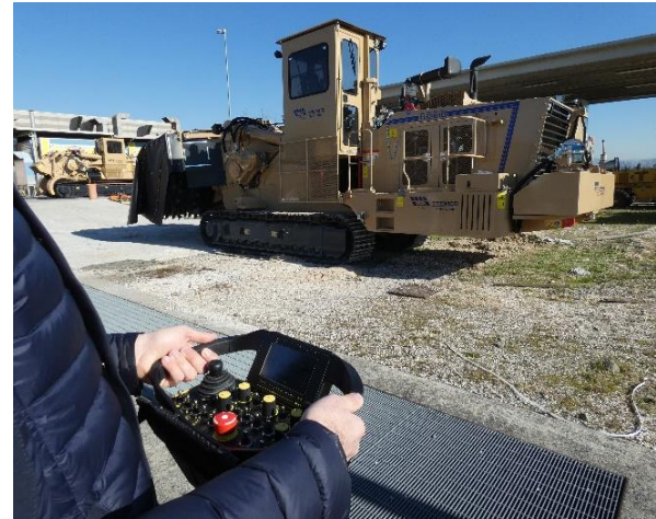
Trencher remotely controlled Available for all TrenchTronic equipped machines
