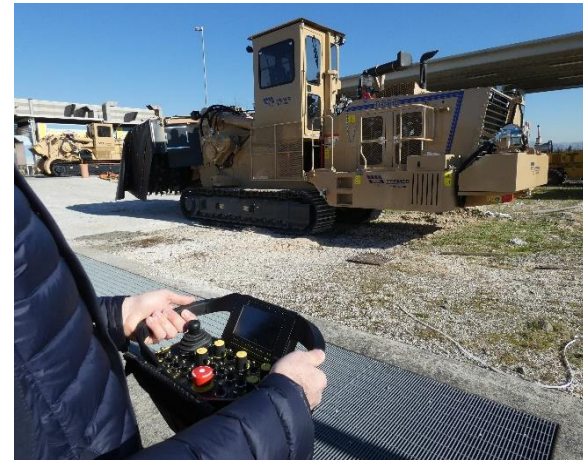
New features, trencher remote control Available for all TrenchTronic equipped machines
