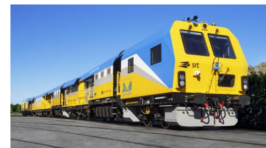
"Vulcano 34M" grinding train
