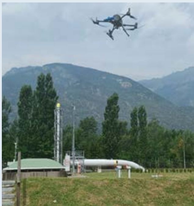
Figure: Methane emission measurement tests using drone-mounted instrumentation
