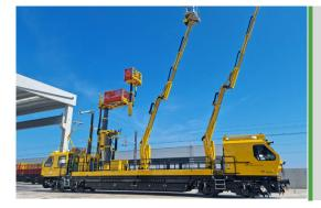
**Egypt - "Green Line" High Speed Rail:** Supply of 2 units model OCPD001, part of the innovative "working train" made of 6 rail vehicles to electrify a new double railway line of 660 km.
