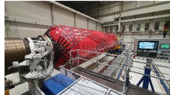
*IMC, Composite case during winding (initial phase)*
