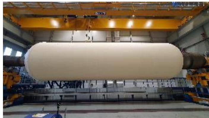
*IMC, Thermal Protection after machining*
