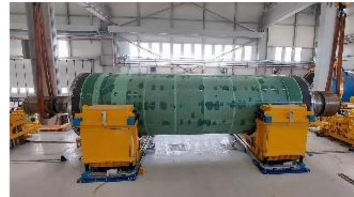
*IMC, Composite case after thermal curing*
